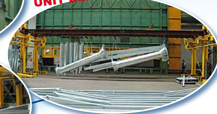
Hot-dip galvanizing – In accordance with DIN EN ISO 1461
